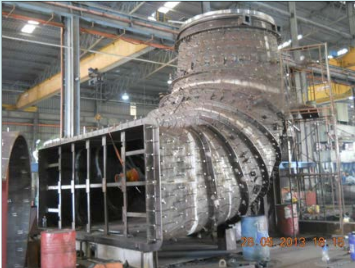
Draft Tube Liner - Completed on June 2013
