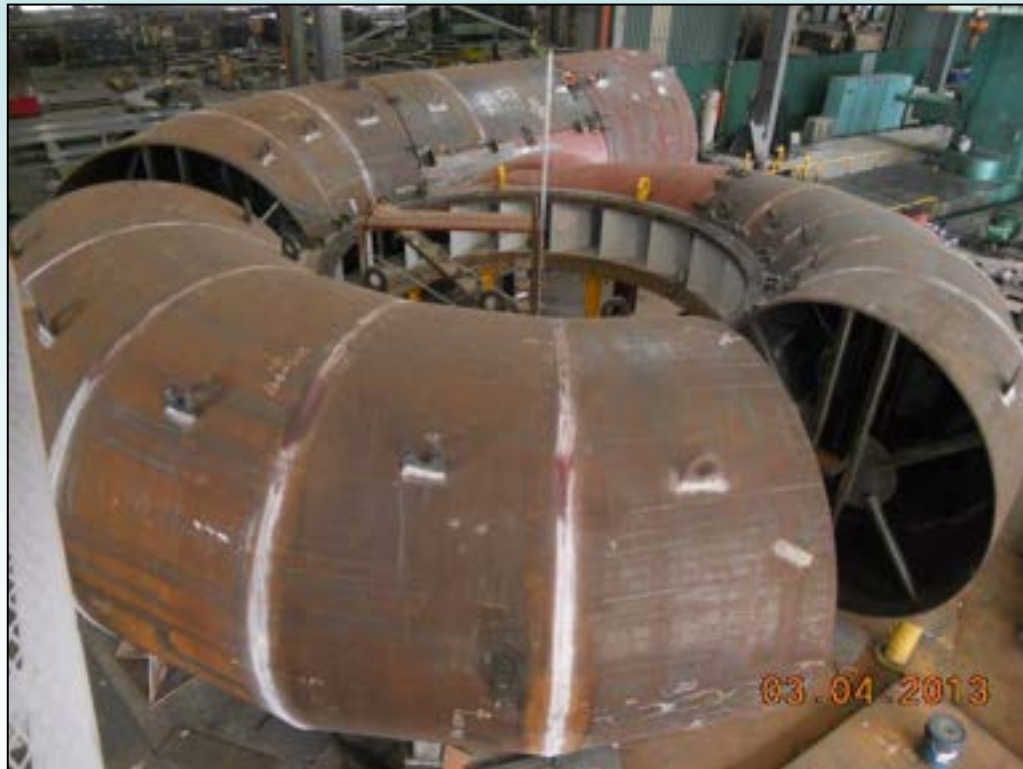
Spiral Case and Embedded Parts- Completed July 2013
