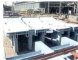
Settler Flash Furnace: Bottom Saddle (300,380 kg)
