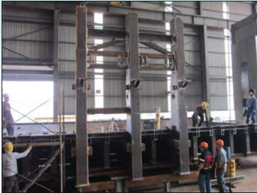
Trial Assembly of Furnace Bottom Plate Saddle
